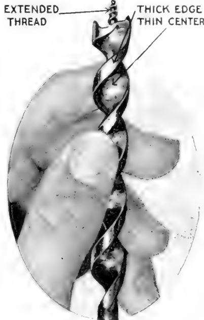
The thread of the bit extends beyond the center of the point
